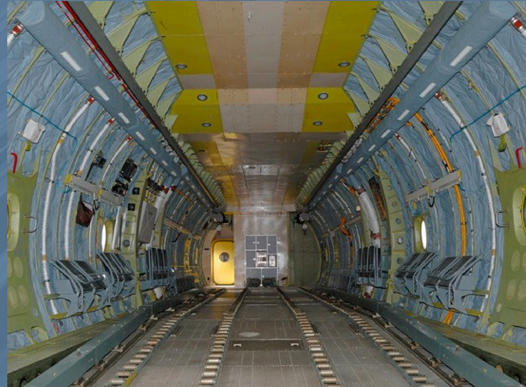
Upgraded Cargo Bay – frame shaped bulk wall Post-Free Design
